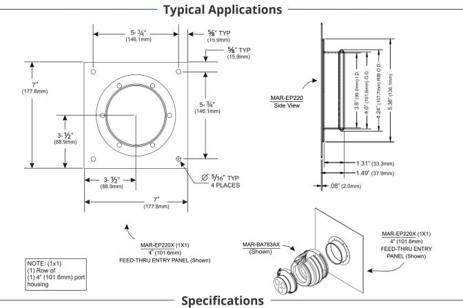
Finish: Entry panels are manufactured from .080" aluminum and are powder coated. All attachment hardware is stainless steel.
